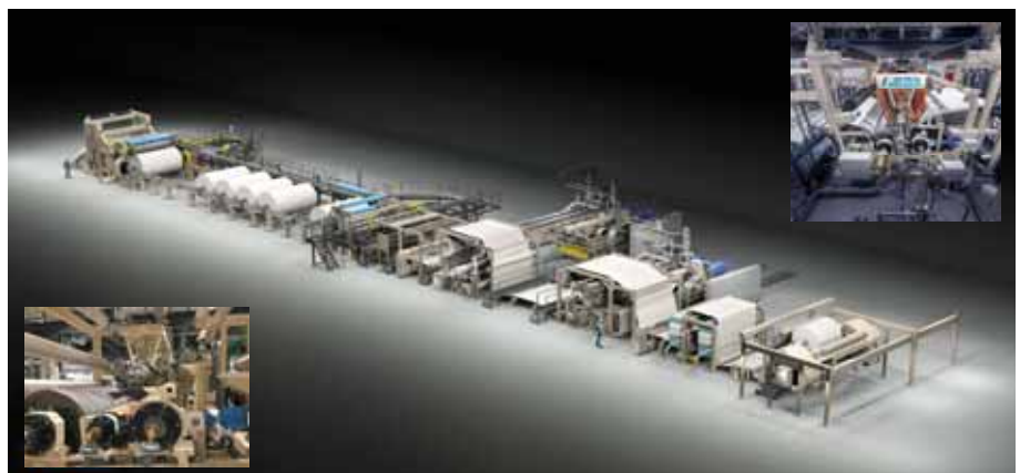
Extrusion coating lines
