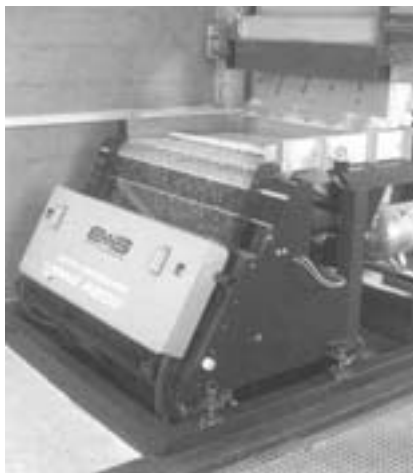
S+S Petmag Metal Separator is said to deliver highest quality and purest recycle
