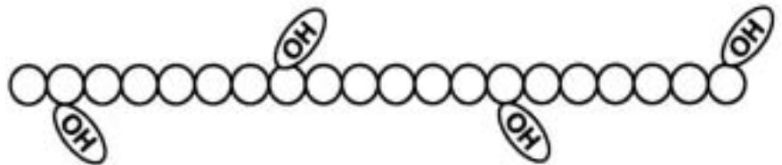
EVAL copolymer: Excellent oxygen barrier. Reduced water solubility.
