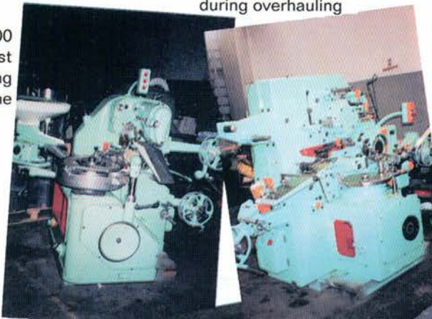
GD 5000 UNI stick wrapping machine during overhauling
